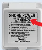
The voltage and amperage should be printed on the outside cover of your existing boat inlet(s)
